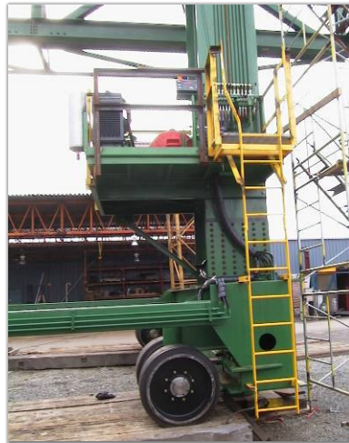
The self-powered hydraulic control centre ran the wheels, steering, outriggers, hoist, trolley and transverse adjustments
