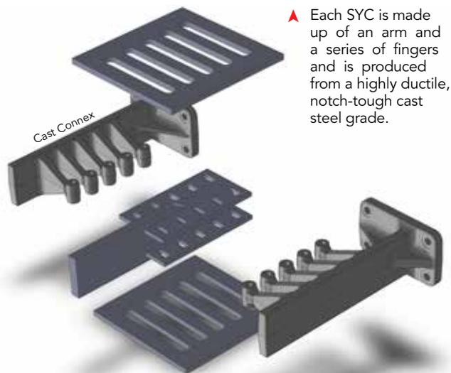
▲ Each SYC is made up of an arm and a series of fingers and is produced from a highly ductile, notch-tough cast steel grade.
